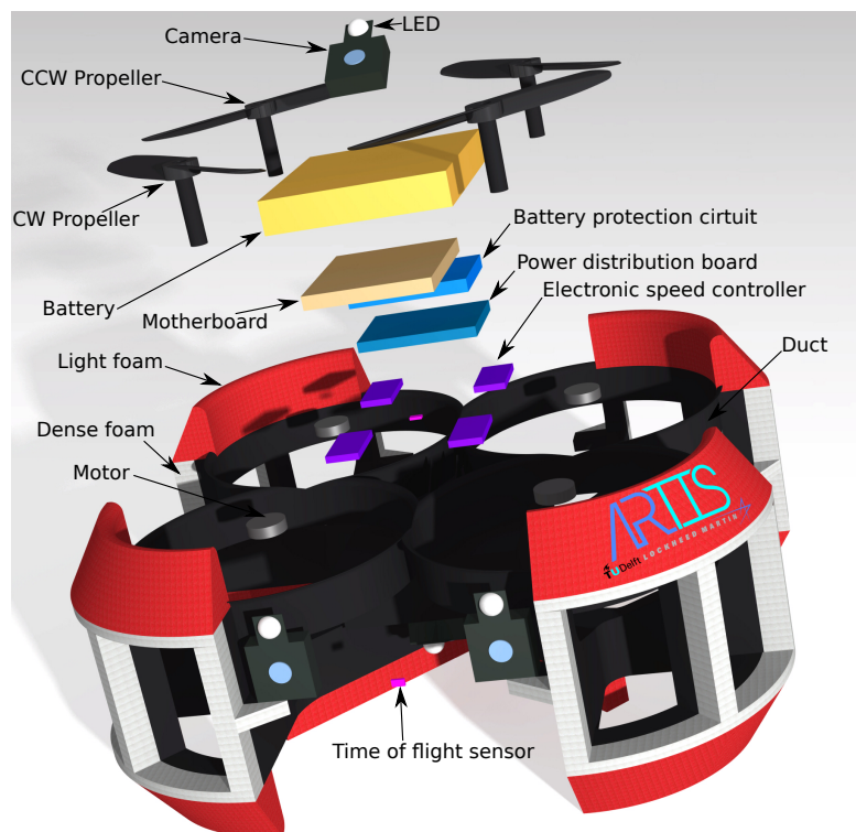
Figure 1: Annotated exploded view of ARTIS
