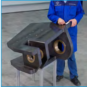
Gear rib of the Affordable Low Cost Aircraft Structures (ALCAS) airliner wing [1].
