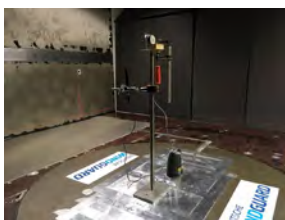
Speaker placed inside the WT, flow-off experiment
