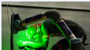
Cyclist mannequin and robot arm with PIV system imaging and illuminating Helium-filled soap bubble seeding
