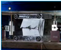
Example of a 40mm thick specimen with a 100J small-mass impact at the point of failure (i.e., 1234kN).
