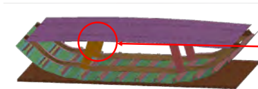
Figure: Global model. Parts connected with rigid ties
