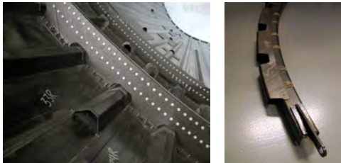
Fig.1: Composite fuselage section mechanically fastened (left) and welded part (right)[1].
