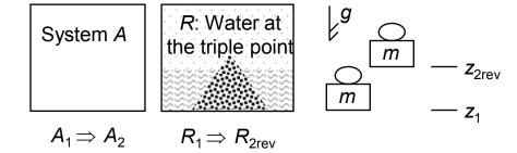
Given any pair of states  $A_1$  and  $A_2$  of a system A (fixed V), make a reversible process for the isolated composite ARm, where m is a weight and R is water at the triple point.
