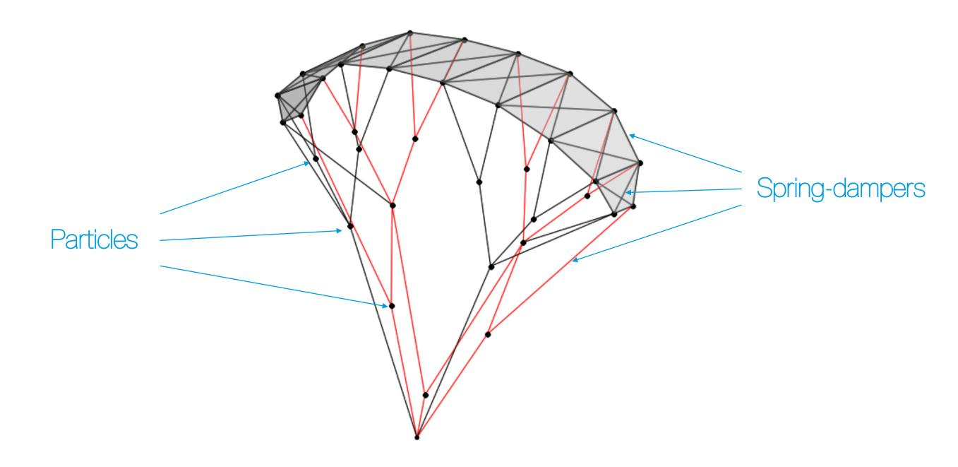
A lift force is applied normal to each panel and scaled based on the plate area and orientation. When simulating turns, this resulted in dynamic stabilization.
