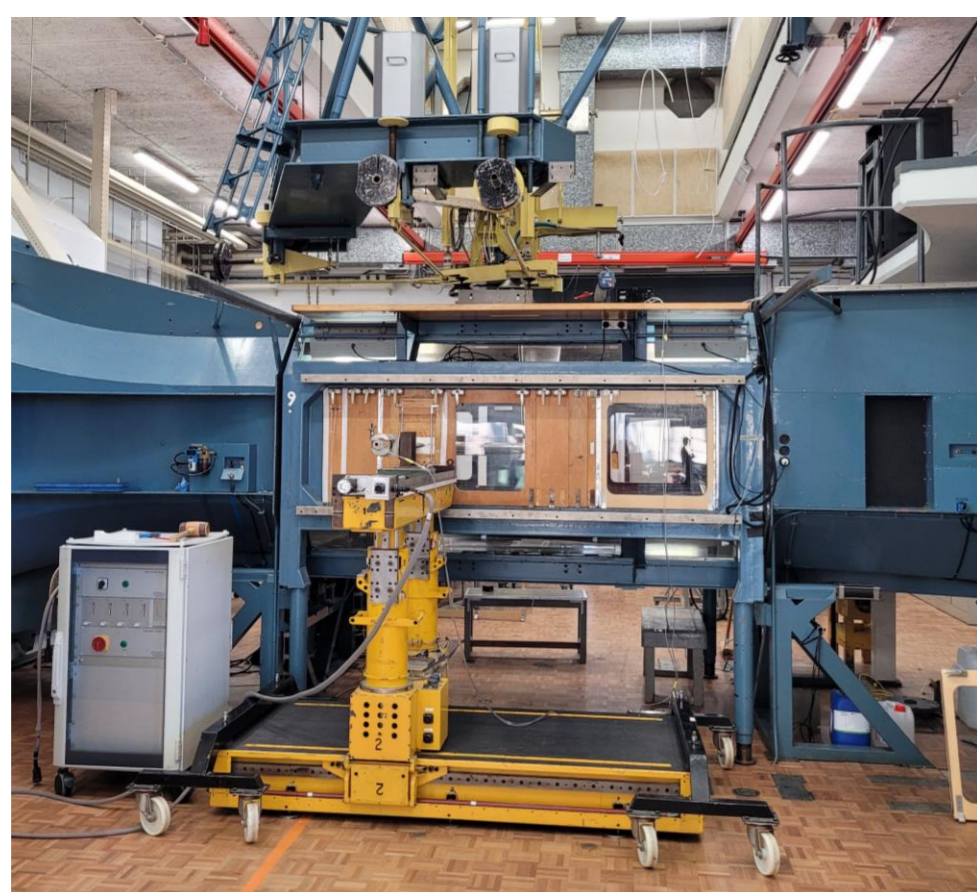
Fig. 3: LTT testing section
