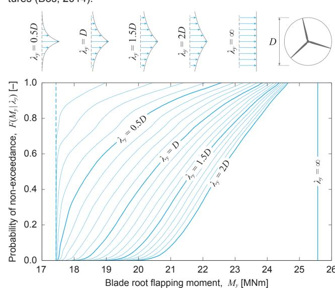
(above) Response of the DTU 10 MW reference turbine to a gust of various sizes. The size of the gust has a large impact on the variation in load output. Smaller gusts have a high probability of triggering no response at all, either by missing the rotor blades or landing close to the blade root. Striking is how even the largest gusts—here 2D is equal to 357 m—remain far below the level of the uniform case.
