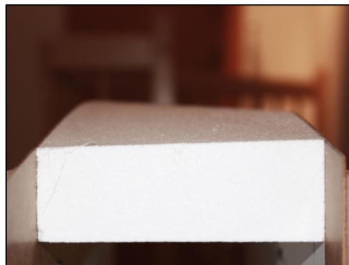
Figure 6.51 - The profiles were arranged at the calculated position with the calculated twist and the wing shape was made with the hot wire cutter as an even ruled surface.
