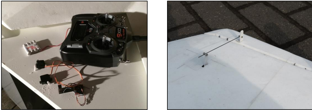
Figure 6.53 – Two servos were installed to actuate the flaps. The battery was installed in the front to place the center of gravity to the calculated position.
