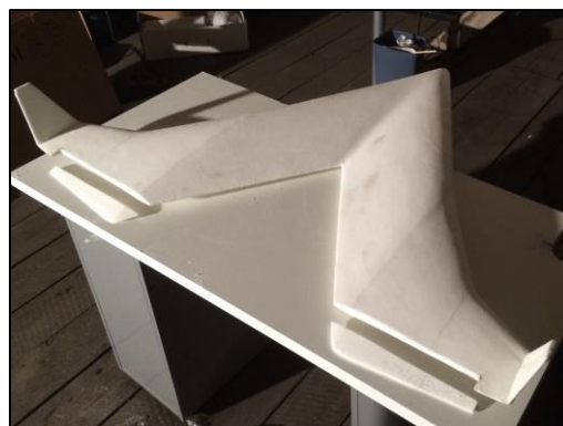
Figure 6.52 – The wings were glued together with styrofoam glue and smoothed with sand paper. The flaps were cut out and the model was covered in a thin layer of glass fiber.
