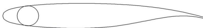
Figure 5.3 – Inefficient use of space with a circular pressurized section placed inside of an airfoil
