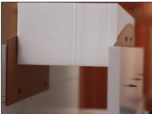
Figure 6.51 - The profiles were arranged at the calculated position with the calculated twist and the wing shape was made with the hot wire cutter as an even ruled surface.
