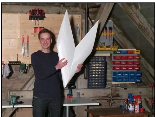
Figure 6.52 – The wings were glued together with styrofoam glue and smoothed with sand paper. The flaps were cut out and the model was covered in a thin layer of glass fiber.
