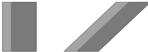
Figure 5.6 – When the wetted area is kept the same the cabin area will increase for higher sweep angles
