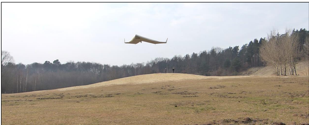
Figure 6.55 – The model was thrown from a little hill out of a height of roughly 3.5m. After a short and fast decent to gain speed after the throw a straight glide path could be taken up on which the Flying V flew roughly 90m. The airplane was easy to control and landed smoothly.
