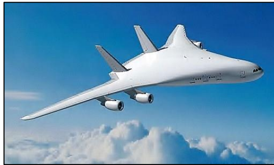
Figure 2.2 – Blended Wing Body concept, EU project NACRE, 2008 [7]
