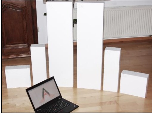
Figure 6.50 - Blocks for the wing elements were cut with a hot wire cutter and the profiles were cut out of wood.
