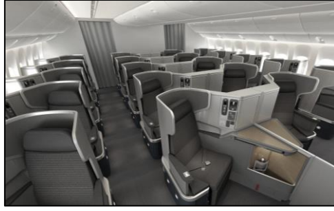
Figure 6.4 – Cabin concept with oblique seats as it is for instance used on Boeing 777 aircrafts of Delta Airlines, picture from [30]
