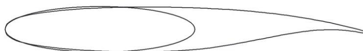
Figure 5.4 – Efficient use of space with an elliptical section inside of an airfoil
