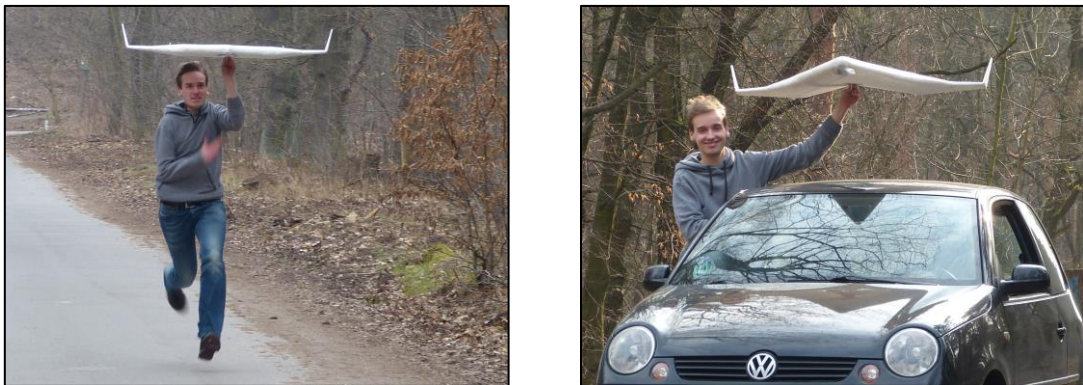
Figure 6.54 – The glider model weighs 770g and has a wing area of 0.43m 2 . To achieve the design C_L=0.25 a speed of roughly 40km/h is required. After first slower tests with running the model was brought up to 40km/h with a car. The rudders were tested and the model seemed well trimmed for a neutral flap position at this speed and stable.
