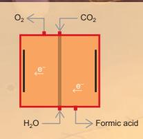
Formic acid is currently almost exclusively produced on the basis of fossil fuels. Previously it was demonstrated on a laboratory scale that it is possible to produce formic acid through direct electrochemical conversion of CO<sub>2</sub> at the cathode. Oxygen is produced at the anode.
