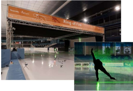
Figure 5. Ring of Fire setup in the skating rink of Thialf, the Netherlands. An athlete skating through a cloud of helium filled soap bubbles illuminated by laser light.
