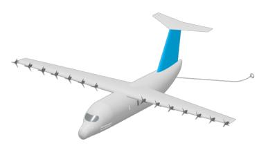
tive process. It features a distributed propulsion system with 14 EMRAX motors to maximise efficiency, with the concept of regenerative propellers to gain energy during the descent phase, while eradicating the need for spoilers. The aircraft structure, integrated with sensors from the manufacturing phase, highlights the use of carbon fibres + PEEK, a thermoplastic with excellent thermal and mechanical properties.
