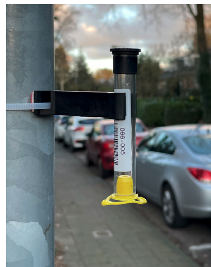
Figure 2 Low-tech: Measuring NO 2 with a Palmes tube mounted on a lamppost.
