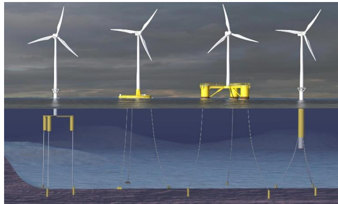
Figure 1: Different foundation options for offshore floating wind turbines. Modified from [4].
