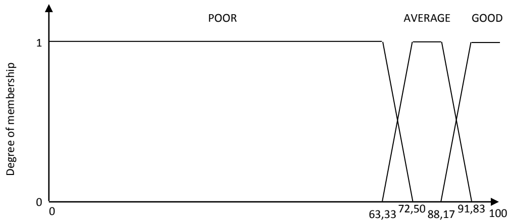
Figure 10. MFs for trust KPI CostRange with overlapping input ranges, and input ranges with a gap.
