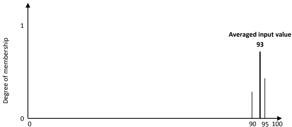
Figure 9. Distribution of input values for poor by the experts for the trust KPI ContractualCost with two of five times the input value 90, and three of five times the input value 95.
