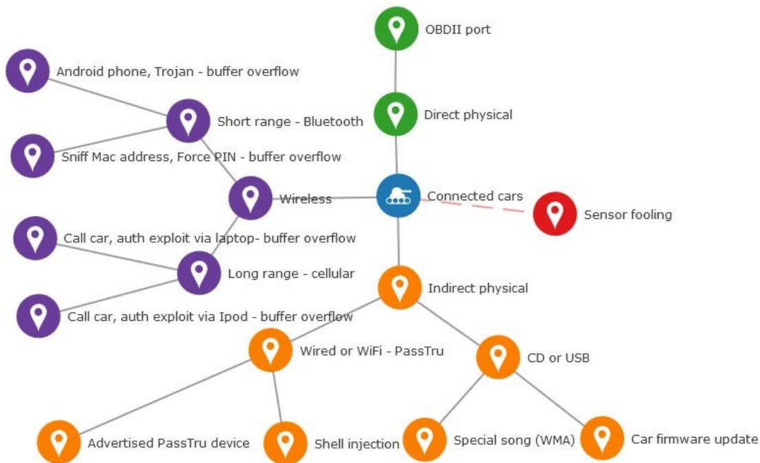
Fig 11. Overview of the clustered attack vectors of a connected car based on research by Checkoway, et al., 2011 and the TU Automotive report 2016.
