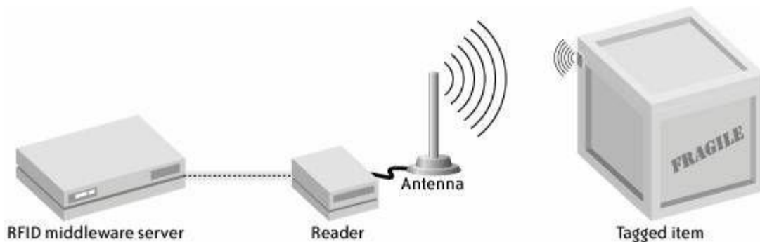
Figure 9: The Workings RFID Technology (Glover and Bhatt 2006)
