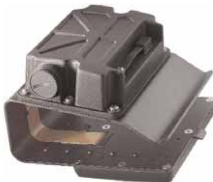
Figure 29: Savi Networks RFID tag [Savi Networks Tag, 2007]
