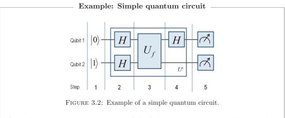
A simple quantum circuit consisting of the following operations: 1. qubit initialization, 2. single-qubit gates, 3. two-qubit gate, 4. single-qubit gate, 5. a measurement.
