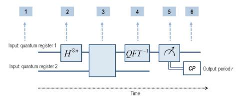
FIGURE 3.4: Example of a gate implementation of Step II of Shor's algorithm, derived from [25, 26]. CP refers to Classical Post-Processing.
