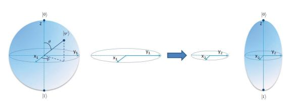
FIGURE 2.3: Visualization of phase damping. On the left the Bloch sphere without phase damping effects, the xy-plane forms a perfect unit circle. On the right the Bloch sphere with phase damping effects, the xy-plane is not forming a perfect unit circle.
