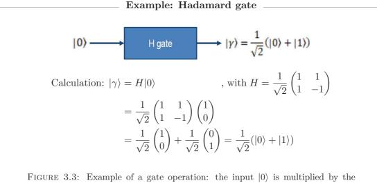
FIGURE 3.3: Example of a gate operation: the input  $|0\rangle$  is multiplied by the Hadamard transform implemented by a Hadamard gate. This produces an output in superposition:  $\frac{1}{\sqrt{2}}(|0\rangle + |1\rangle)$ .
