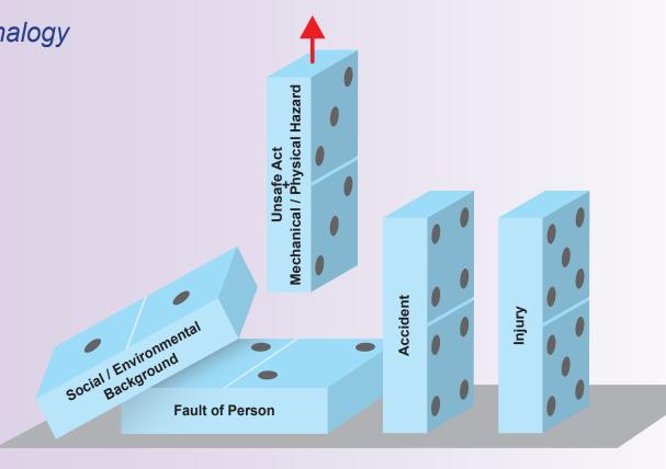
Removing the central factor disrupts the accident sequence
