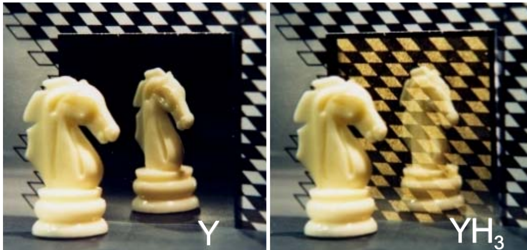
Figure 1.5: Appearance of a 500 nm thick Y film covered with 20 nm of Pd before (left) and after (right) exposure to 10^5 Pa of H_2 at room temperature [11].
