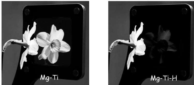
Fig. 1.3. Mg_{0.7}Ti_{0.3} thin film in the metallic (left) and in the hydrided (right) state during hydrogenation [2].
