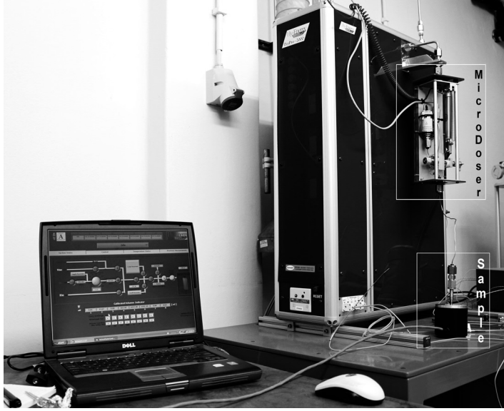
Fig. 2.1. PCTPro-2000 Sieverts apparatus (Hy-Energy LLC) with MicroDoser attachment and the sample holder.
