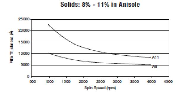
495PMMA A Resists
