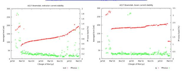
This increment in instability is a strong indication that the filament is approaching its end-of-life. Last November, I for the first time noticed the instability, but it recovered, and by then a new filament on the EBPG5000Plus seemed more necessary, which was installed in December.
