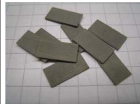
cut and homogenized plates ca. 12x6x0.6 mm
