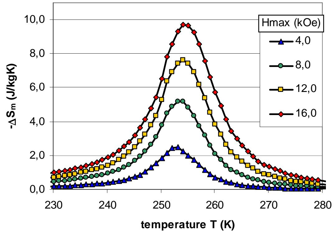
$$\begin{aligned} \rho &= 7.24 \text{ g/cm}^3 \\ -\Delta S_m @ 16 \text{ kOe} &= 67 \text{ kJ/m}^3\text{K} \\ T_{\text{peak}} &= -19 \text{ }^\circ\text{C} \\ \Delta T_{\text{WHH}} &= 14 \text{ K} \end{aligned}$$
