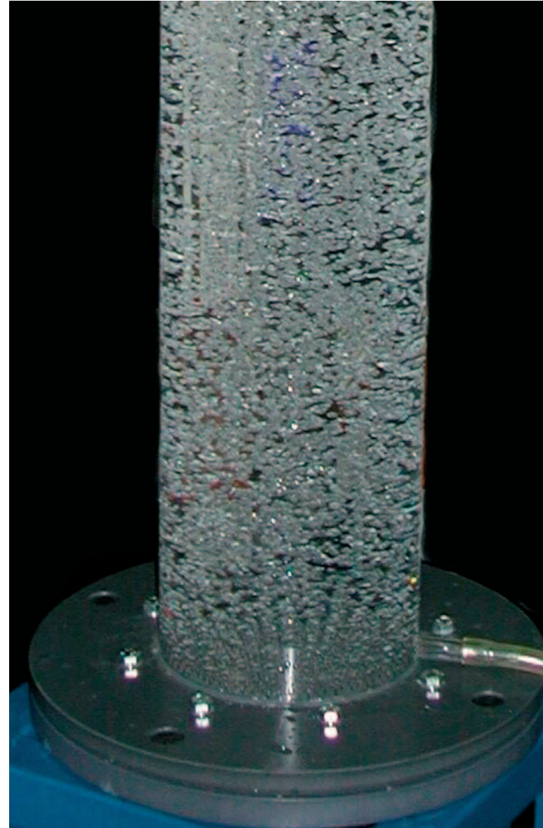
A bubble flow with a gas fraction of fifty-five percent can still be non-turbulent.
