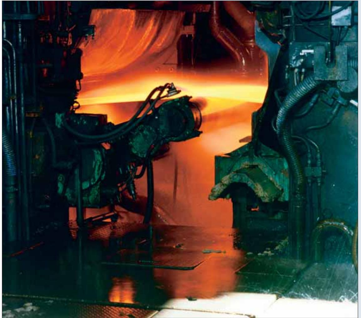
At the Corus IJmuiden mills, steel at 1200 °C is rolled at high speed to the desired thickness in a number of steps, then cooled with water.
