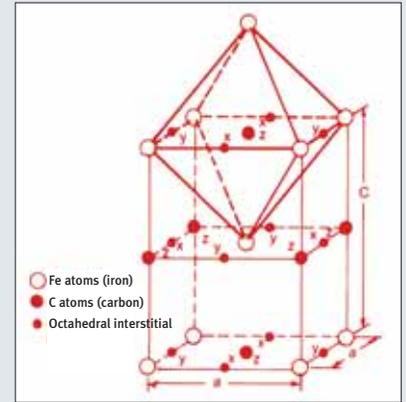
The crystal structure of martensite is very similar to that of ferrite. The difference is that the C-axis of the martensite crystal structure is elongated relative to the base plane (the A-axis) due to the formation process in the presence of carbon, which is frozen in the spaces between the relatively large iron atoms.
