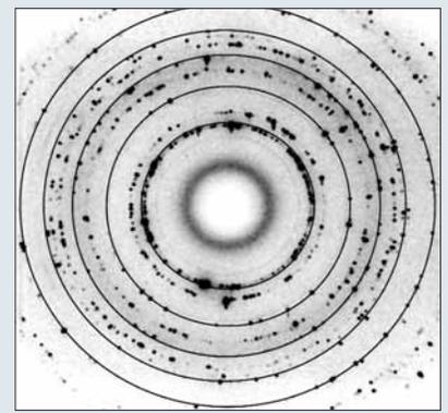
Diffraction pattern of austenite and ferrite. As the steel sample cools, the austenite crystal structure is transformed into ferrite, causing additional dots to appear on the detector (the dots on the circles). This enables the observer to see live when a crystal of the new ferrite phase is being produced. The growth of the crystal can subsequently be determined by making a film of a large number of diffraction patterns and converting the intensity of a dot into crystal size.
