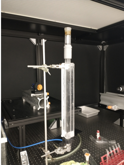
Figure 3.1: The measurement column with filter attached.
