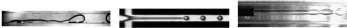
(a) Jet Flow observed by Fu et al [46] (b) Jet Flow observed by Cubaud et al [45] (c) Deformed Interface flow observed by Kashid et al [27]
