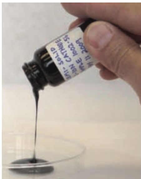
Figure C.1: An example of the suspensions used in Duduta et al. (2011). The fluid semi-solid suspension contains \text{LiCoO}_2 powder as the active material and Ketjen black as the conductive material, dispersed in alkyl carbonate electrolyte. The respective volumes and concentrations are unknown. [13]
