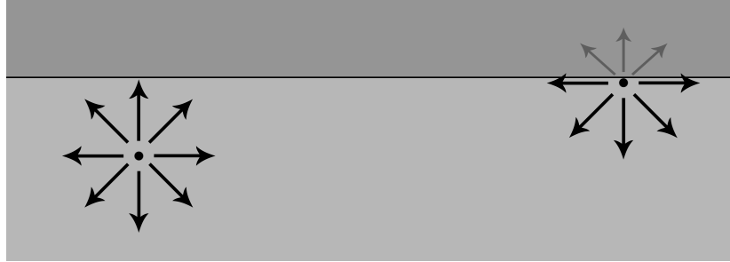
Figure 1: Schematic representation of surface tension forces acting on a molecule. The boundary between the interfaces is shown as the black line. The dark gray mass above the boundary is either a solid or a liquid, the lighter gray depicts a liquid. The arrows represent cohesive forces between the molecules and their neighbouring molecules.
