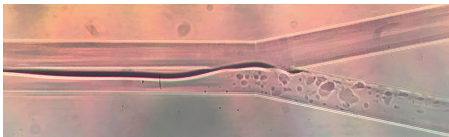
Figure 9: A photo showing the wetting of the organic channel by the aqueous phase, making aqueous leakage into the organic outlet more plausible. It was taken at a flow rate of 30\mu\text{l}/\text{min} for both the organic and the aqueous phase. The organic phase depicted is decane.
