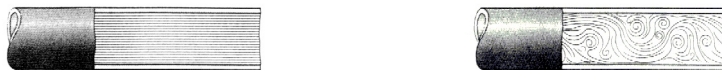
(a) Parallel flow lines at laminar flow regimes. (b) Unstable flow lines at turbulent flow regimes.
