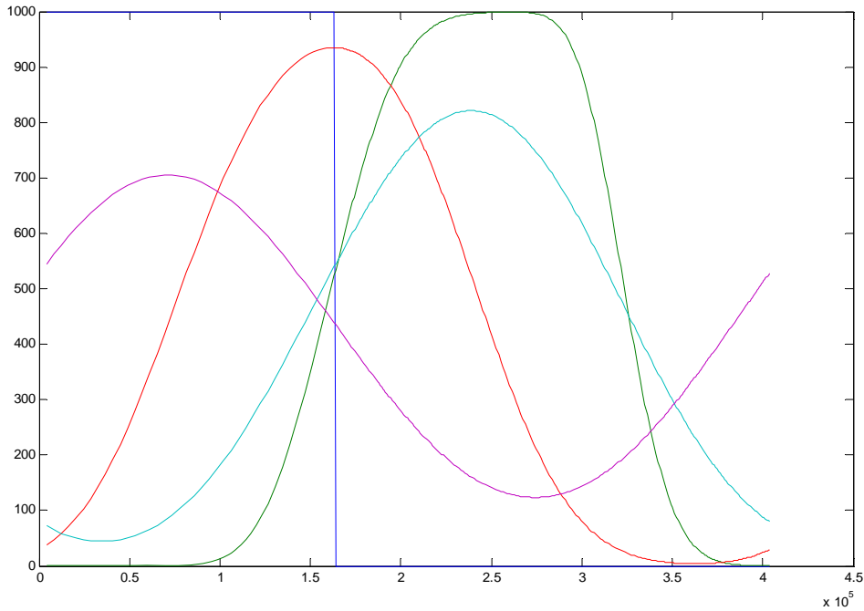
Figure 9.2: Precursor concentrations ( \#/cm^3 ) set out against the relative “Volume position”. For different times: t=0 s (blue), t=10 (green), t=30 (red), t=60 (cyan), t=100 s (purple), with no decay in time of the precursor.
