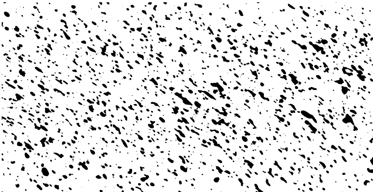
Figure 3.7: Bubbles inside the loop after processing picture. Liquid flow = 037L/s and gas flow = 5cm 3 /min
