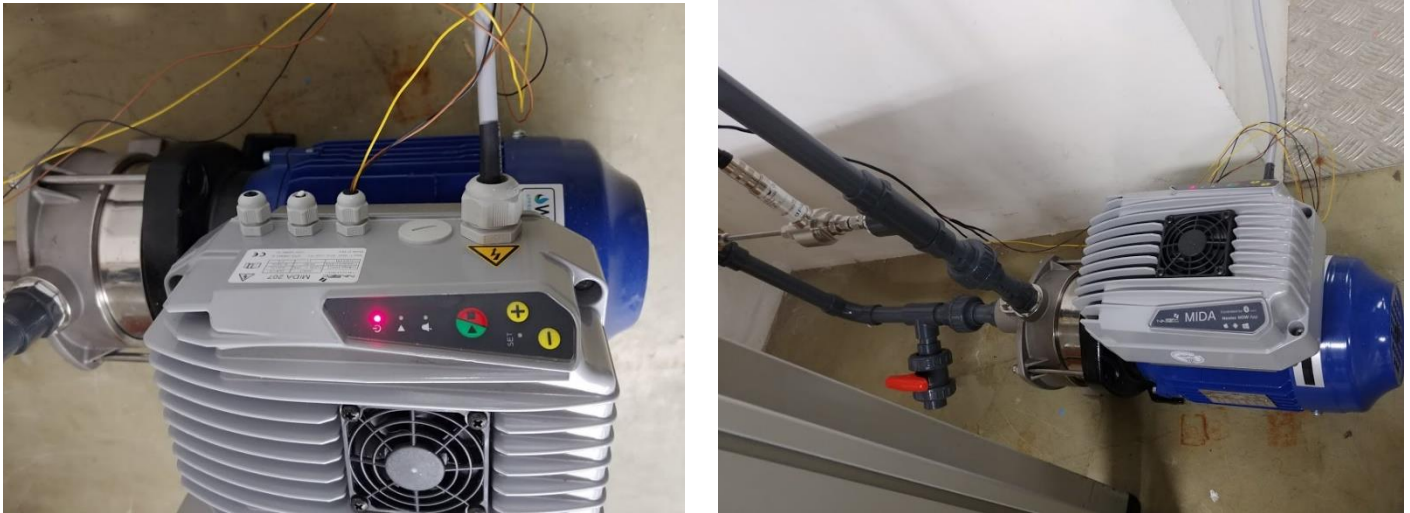
Figure B.1: The Nastec Mida pump, which introduced movement to the liquid.
