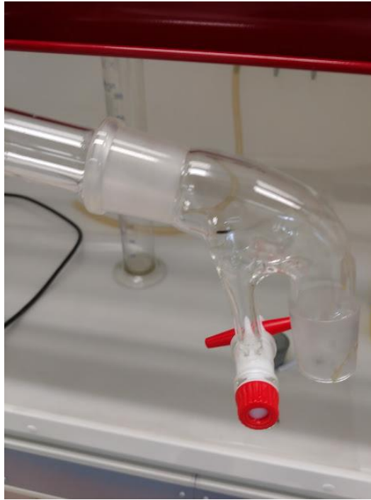
Figure 3.4: The used Hallimond tube to capture the particles with and the bend tube that was placed on top of the Hallimond tube to enlarge its capacity.
