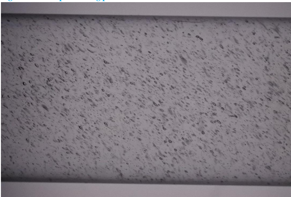
Figure 3.6: Picture of the bubbles generated in the loop. Liquid flow = 044 l/s and gas flow = 10 cm 3 /min
