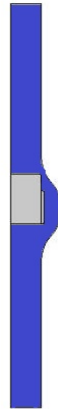
Figure 3.3: Two-dimensional axisymmetric model of the freeze plug with a pipe added before and after the plug part. In the model, the pipe before and after the freeze plug is made extra long in order to let the velocity profile recover from the freeze plug.
