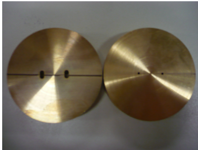
Figure 3.2: The two collimators used in the experiments with. Left the 2 [mm] collimator and right the 1 [mm] collimator.
