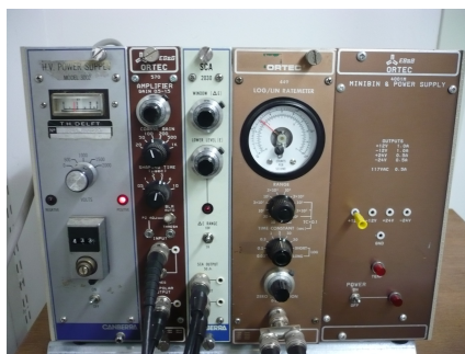
Figure 3.5: A picture of the amplifier (second slot) and the SCA (third slot)
