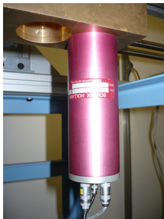
Figure 3.4: The scintillation detector used in the experiments
