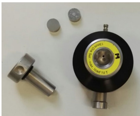
Figure 2.4: The die used to prepare the pellets for IR-spectroscopy.
