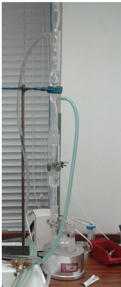
Figure 2.7: Experimental set-up of the Soxhlet leaching test.
