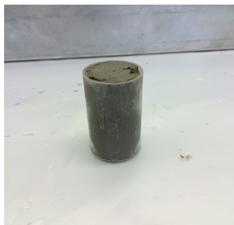
Figure 34: Saturated claycore in a polycarbonate vial.
