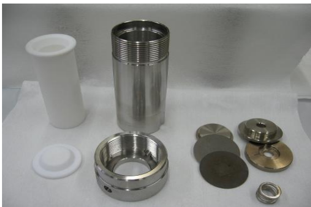
Figure 4 Different compartments of typical autoclaves used for hydrothermal synthesis
