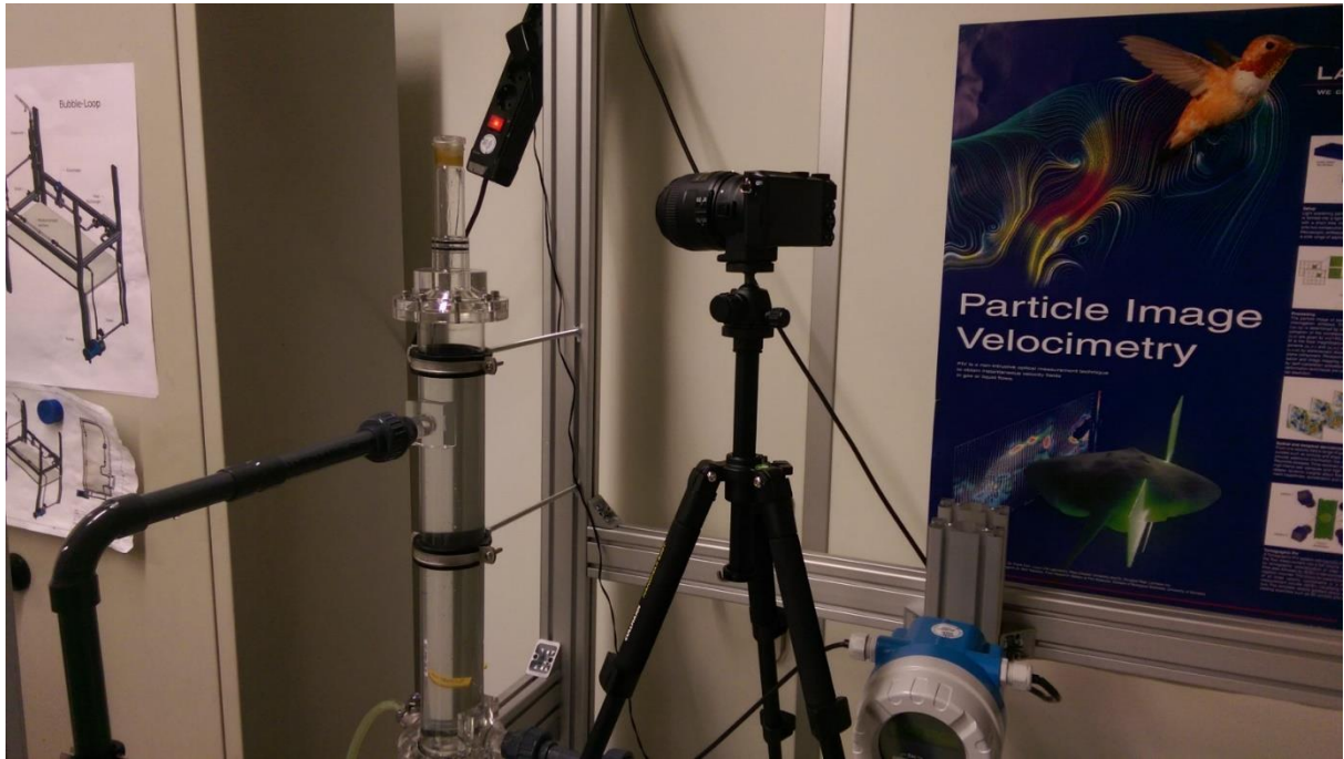
Figure 8. Setup for the gas holdup measurements.
