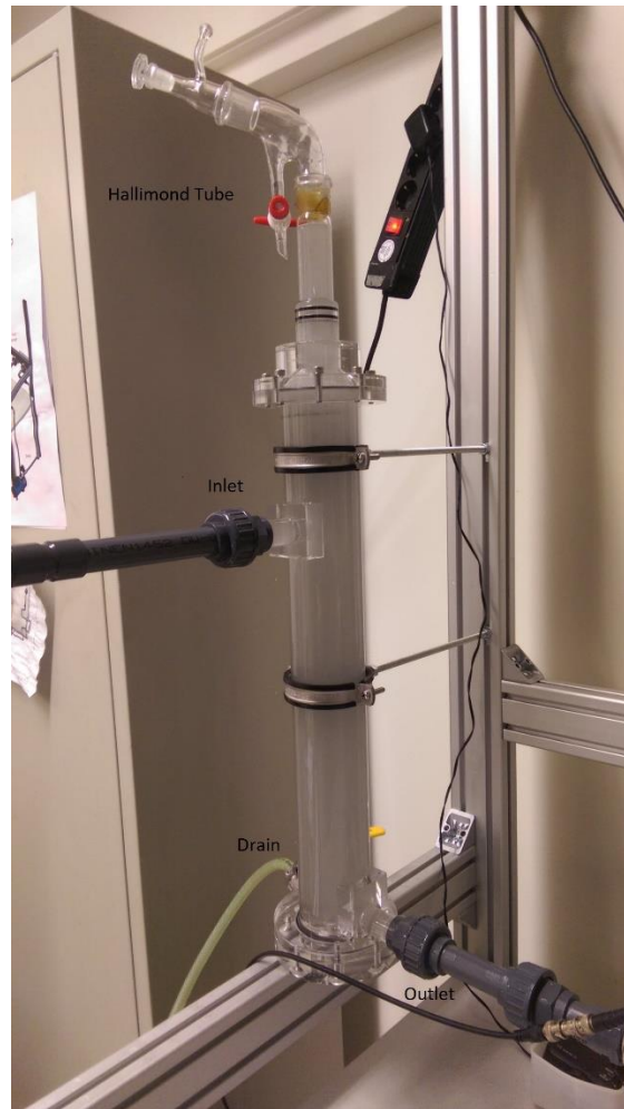
Figure 6. The flotation column and the top mounted Hallimond tube.
