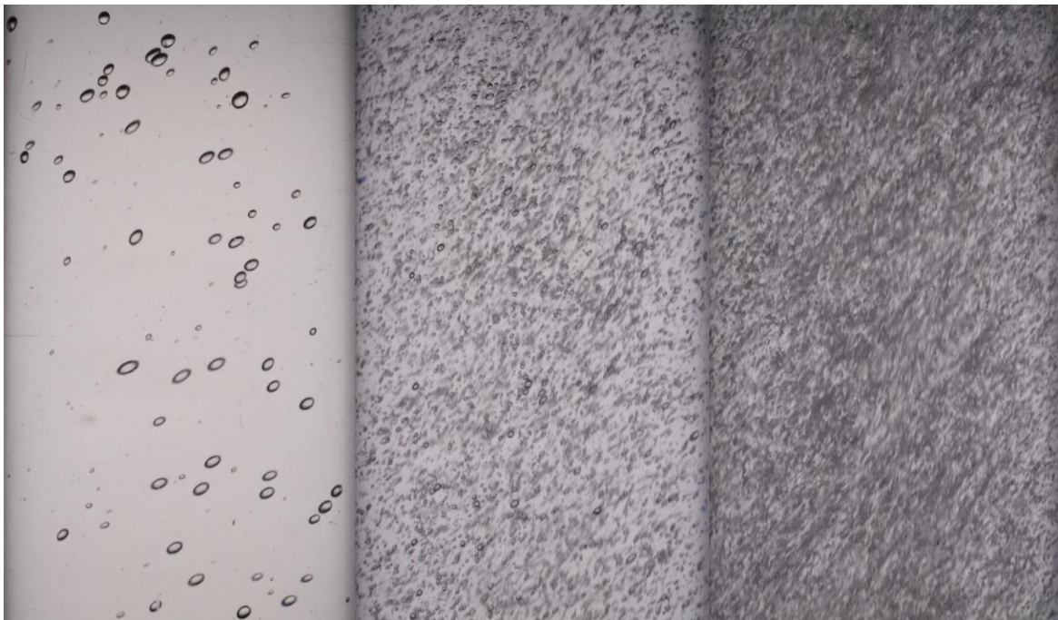
Figure 19. Example images of bubbles for three different fluid flow rates at a fixed gas flow rate of 10 \text{ cm}^3/\text{min} . From left to right: 0.14 \text{ l/s} , 0.35 \text{ l/s} and 0.58 \text{ l/s} .
