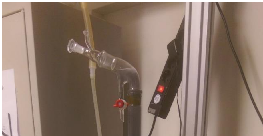
Figure 9. Particle extraction experiment right after adding the particles and mounting the Hallimond tube.
