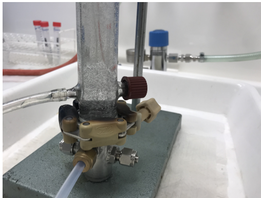
(b) bottom of the column. On the left the tube connection to extract the content of the column can be seen. Also the flange connection to the bubble distributor can be noticed.
