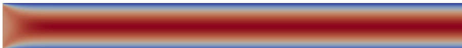
Figure 4.3: The fluid velocity in the flow direction, red indicates high velocities, blue indicates low velocities
