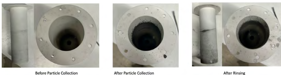
Figure A1: 500 nm nickel particles before particle collection, after particle collection, and after rinsing.
