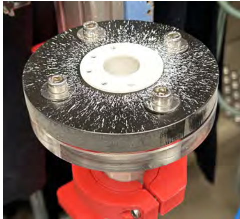
Figure A2: 10\ \mu\text{m} of zinc-oxide with 7.5\ \text{mm} collector and inlet diameter of 1\ \text{mm} at volume flow of 300\ \text{cm}^3 \cdot \text{s}^{-1} . Many particles were ejected out of the column, leading to an underestimation of particles recovered.
