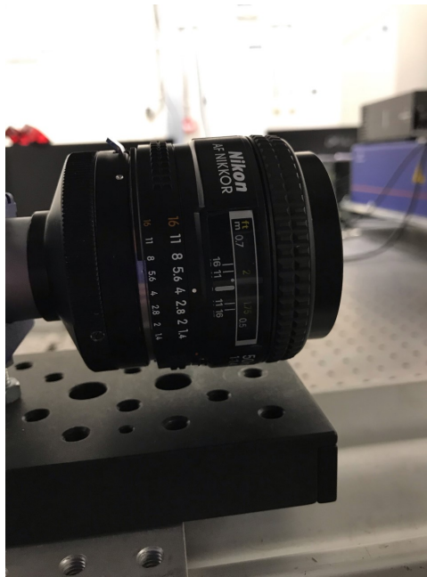
Figure 15: Detector used for grabbing high-speed images. On the camera (right-hand side) a filter can be mounted that detects LIF-active particles.
