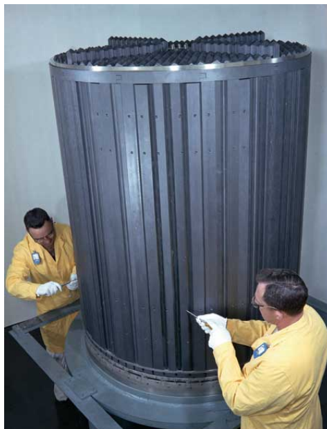
Figure 1.8: The core of the MSRE reactor. Unlike the Molten Salt Fast Reactor, the MSRE used a moderated reactor core, this one is made of graphite channels through which the fuel salt flowed.
