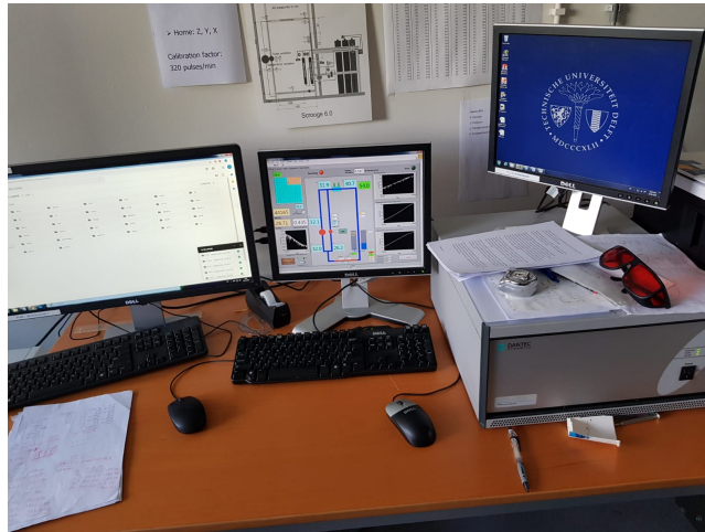
Figure 3.5: Picture of the PC's which are used to control the setup (middle and right screen) and run the BSA Flow software (left screen) [38]. The processor is located beneath the right screen.
