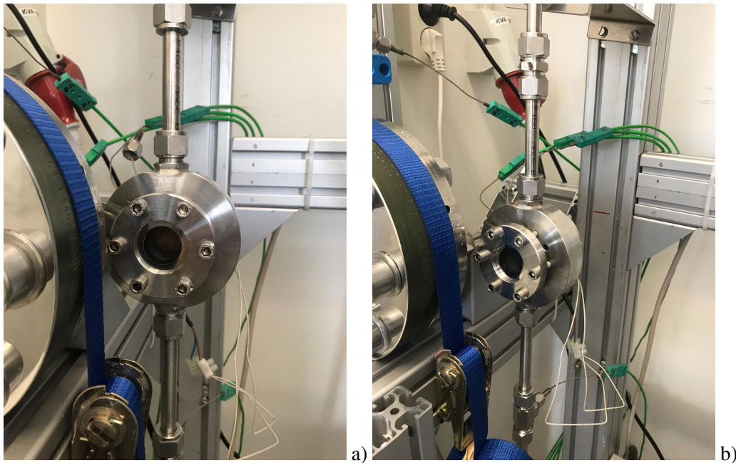
Figure 3.3: Pictures of the window in the Scrooge 6.0 setup. A cylinder is held by a copper backside with heating elements incorporated and a front glass plane to give optical access to the freon. The green wires are the thermocouples wires which are connected to the thermocouples in the copper backside. To the left of the window is the Serpentine located, which is part of another study. ©Y. Zheng
