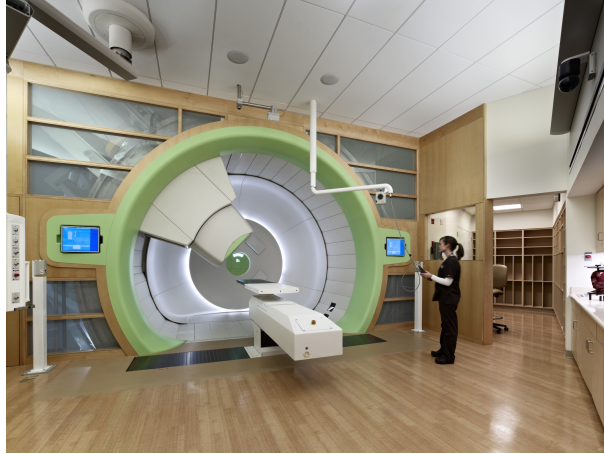
Figure 1.2: A proton therapy treatment facility [5]. The patient is placed on the couch, which can be shifted to perfectly align with the gantry. Both the couch and the gantry can be rotated during treatment to make dose delivery from different angles possible. Immobilization devices are used to keep the patient fixed in space during both imaging and dose delivery.
