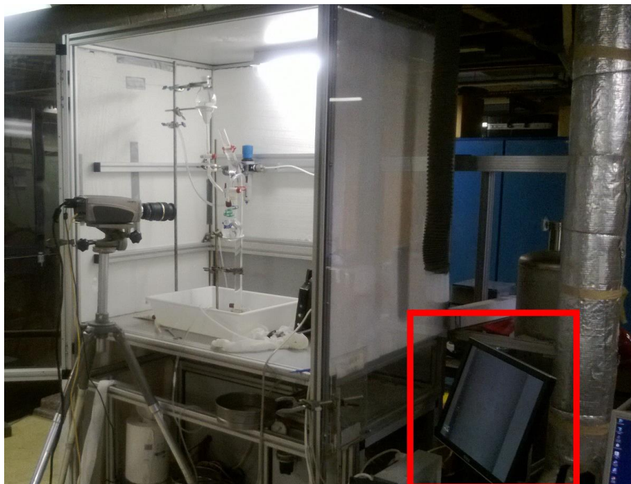
Figure 4.11. A picture of a high speed camera which is filming the process. The red square indicates the display which shows the live image of the camera.
