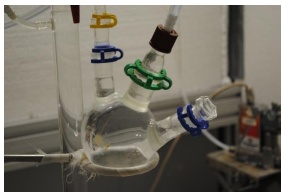
Figure 4.6. A three-neck flask is connected to the Hallimond tube. The three-neck flask is used to collect the particles that are floated to the surface by the gas flow. The first neck is connected to the Hallimond tube. A tube is connected to the second neck to release the air inside the flask during the filling of the set-up. The third neck is sealed with a plug.
