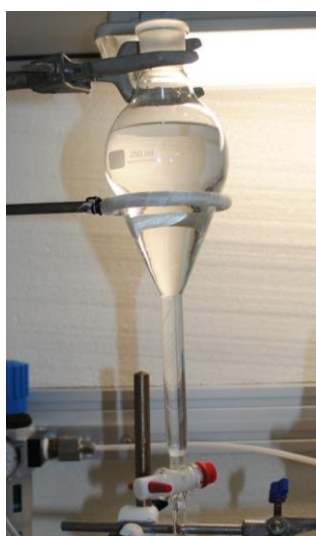
Figure 4.7. The separatory funnel is used in the set-up to add the particles to the column. The valve can be opened and closed by hand. The funnel is filled with a liquid and the weighted particles are added to the funnel, while the valve is closed. When the particles are settled at the bottom the valve can be opened to add the particles to the column.
