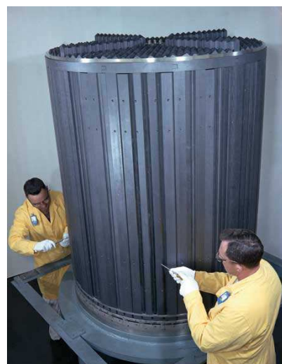
(b) The MSRE graphite core.
