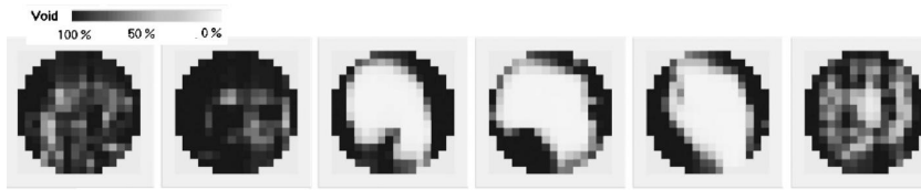
Figure 3.5: The measurement of a gas bubble with a wire-mesh in a two-phase flow Prasser et al. (2005).
