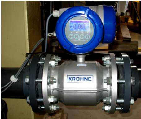
(a) Krohne Optiflux 2300 C flowmeter.
