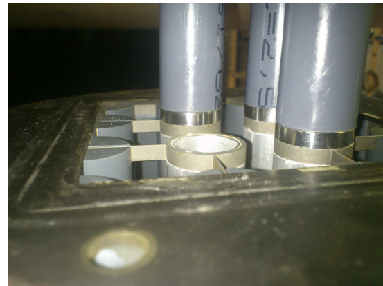
(b) Connection between the PVC and aluminum rods.
