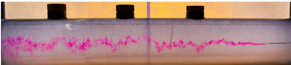
Figure 4.4: A picture of the dispersing purple dye that was injected into the turbulent pipe-flow.
